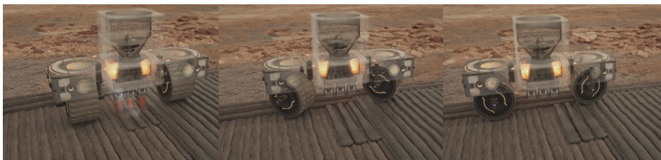
Fig. 12. 3D printing sequence and edge maneuvering
